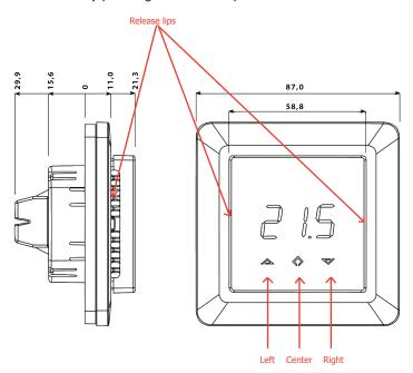
Use e.g. a small slotted screwdriver. The front cover and the frame can now be removed.
