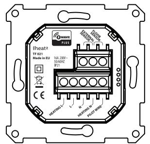
Now connect the wires to the thermostat's terminals:
