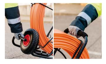
The user may drive easily the resulting trolley using one of the portable configurations: one handle on the front and one handle on the side.
