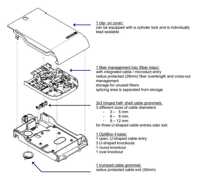
On request, OptiBox 4 is delivered including adapters and connectors. Connectivity components are enclosed as a mounting- kit. Further accessories like splice holder, Patch Cables, Pigtails, Masterline Quick, etc can be included as well, but they have to be ordered individually.
