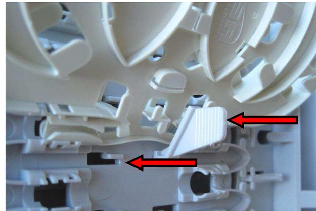
The broken out ACS Cassette Support can be placed in the shown position after using.
